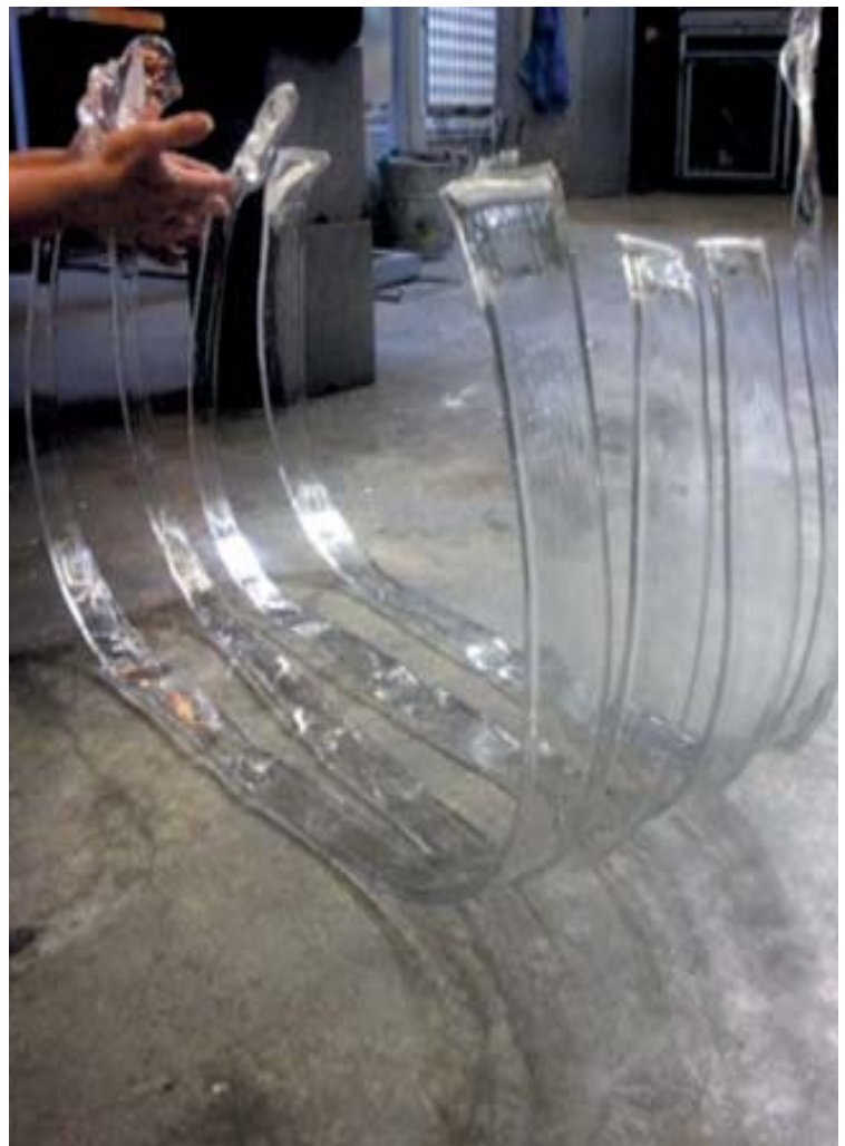
Glass rib forms taken from canoe mold. Photo by Brad Copping
